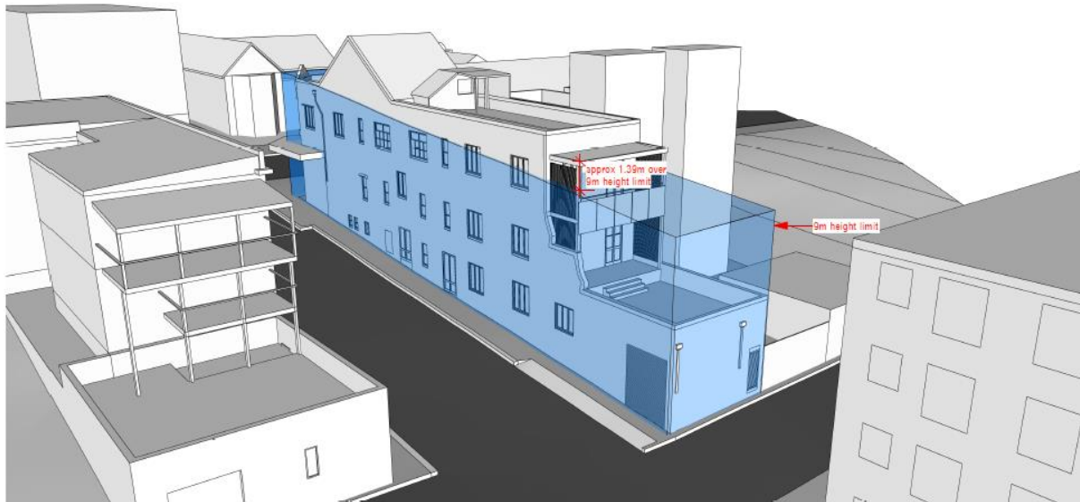
Figure 26: Height plane diagram showing the proposed elements above the 9m height limit
