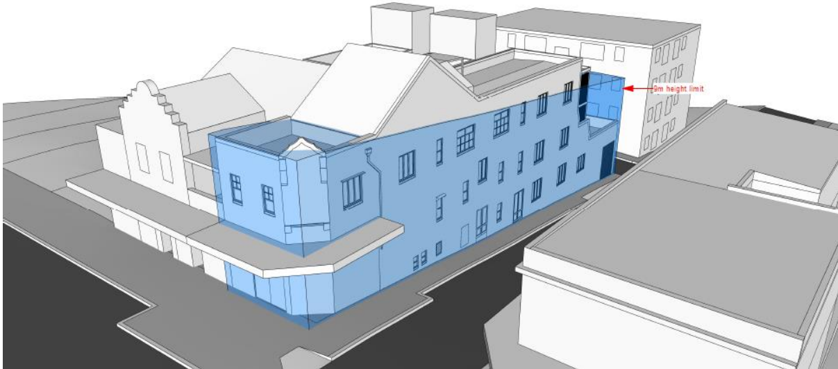
Figure 28: Height plane diagram showing the proposed elements above the 9m height limit
